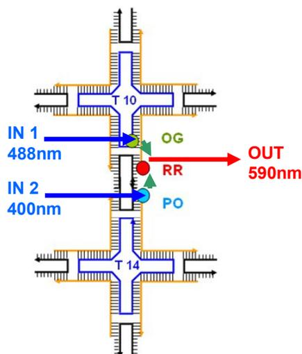
**Figure 6. Schematic of the energy transfer OR-gate.**
