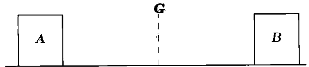
Fig. 23. An equivalent problem. A point robot must be navigated halfway between the blocks A and B . The distance between A and B is not known. The robot has force sensing and a clock. However, it has poor position
