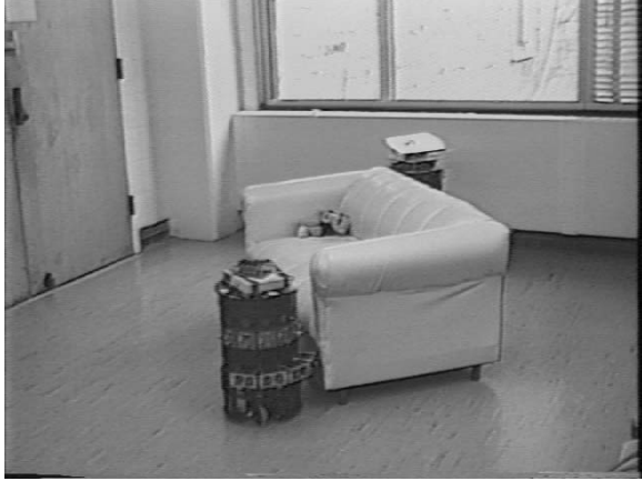
Figure 7: Two mobile robots cooperating to reorient a couch: a snapshot taken from a couch reorientation experiment.
