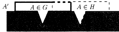
Fig. 13. The set of thick solid edges comprises A' for A \in G . The dashed line outlines the target polygon in the failure region H . The thick dashed line is the overlap region.
