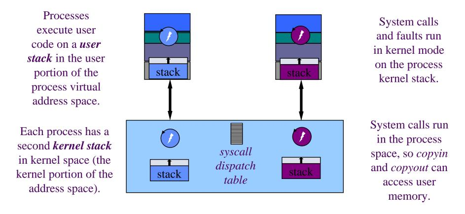
The syscall trap handler makes an indirect call through the *system call dispatch* table to the handler for the specific system call.
