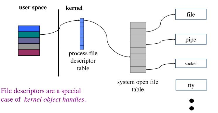
The binding of file descriptors to objects is specific to each process, like the virtual translations in the virtual address space.
