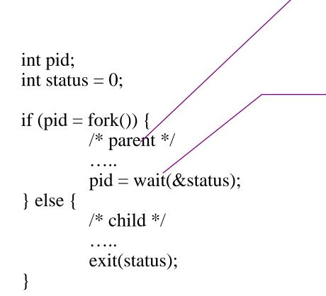
The **fork** syscall returns <u>twice</u>: it returns a zero to the child and the child process ID (pid) to the parent.
