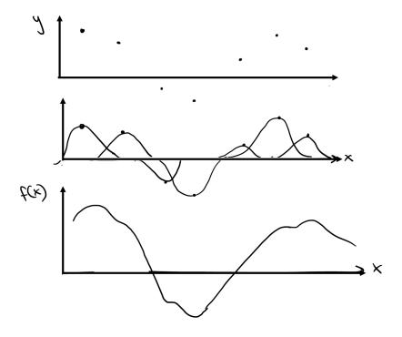
The data is on top. A bump is placed on each point, with height  $y_i$ . These are summed and normalized.
