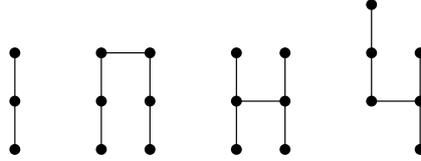
Removing a clause edge from  $M$  transforms a pair of two-edge paths into a barbell in  $G \setminus M$ , which does not increase the size of the maximum matching. ◀
