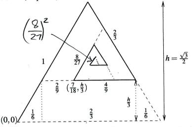
Here one starts at x-y-coordinate (0,0) and goes up at angle  $60^{\circ}$  one unit. Then down at angle  $60^{\circ}$  shrinking the length by a factor 2/3. Then back at angle  $60^{\circ}$  shrinking the length again be a factor 2/3 to length 4/9. The new x-y-coordinate is  $(7/18, \sqrt{3}/6)$ , as indicated. One continues the up-down-back's, always shrinking the line segment lengths by a factor 2/3. Only one more is shown.
