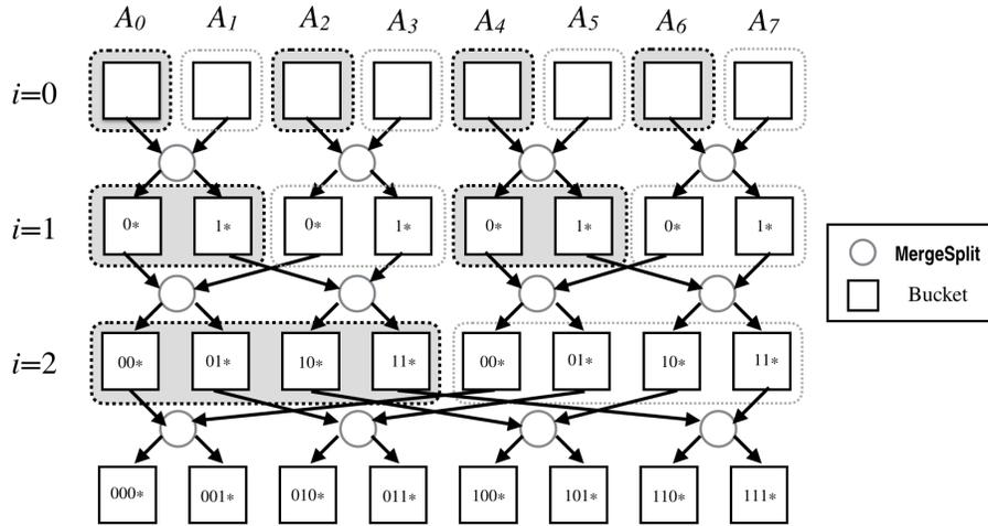
Figure 1: **Oblivious random bin assignment with 8 buckets.** The MERGESPLIT procedure takes elements from two buckets at level  $i$  and put them into two buckets at level  $i+1$ , according to the  $(i+1)$ -th most significant bit of the keys. At level  $i$ , every  $2^i$  consecutive buckets are semi-sorted by the most significant  $i$  bits of the keys.
