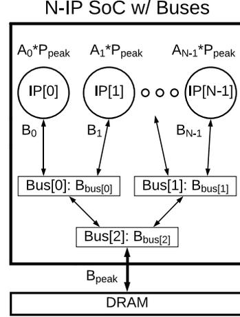
Figure 11: N-IP SoC with detailed interconnect extension.
