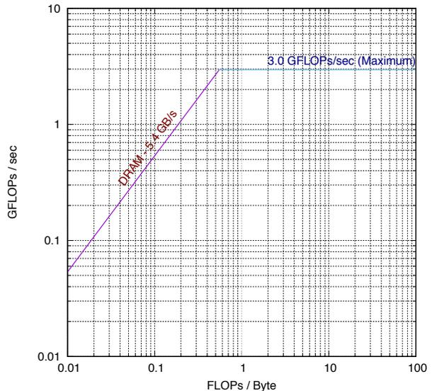
Figure 9: DSP roofline for the scalar threads. The  $y$ -axis scale here is smaller than Figure 7 because we use the HVX scalar engine, and not the high-performance (non-IEEE compliant FP) vector engine (see details in Section IV-D).
