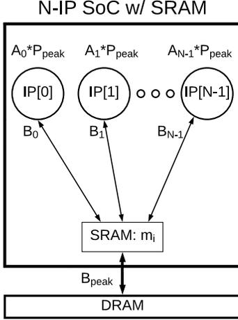
Figure 10: N-IP SoC with on-chip memory extension.
