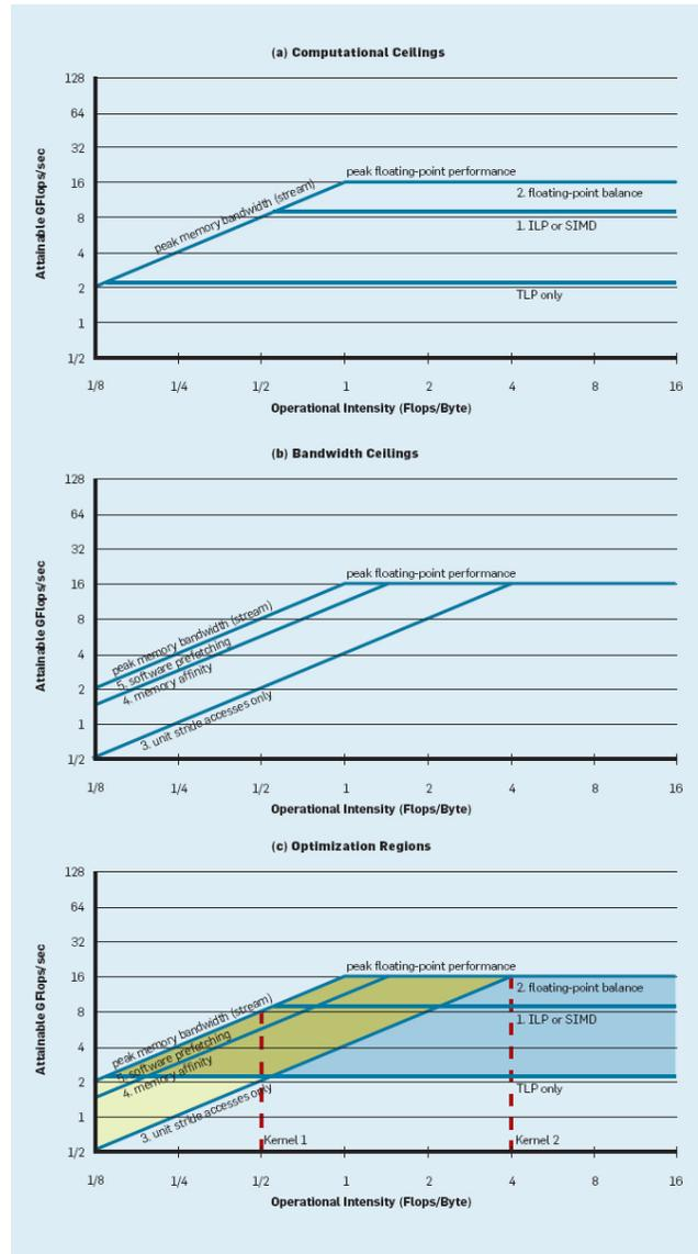
Figure 1: Roofline model [8]. Reprinted with permission.
