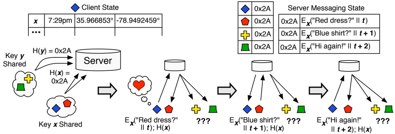
**Figure 1: An illustrated sequence of operations.** Let  $H$  denote a cryptographic hash function and  $E_x(m)$  denote the encryption of message  $m$  with key  $x$ . Encounter keys  $x$  and  $y$  hash to the same value, leading the server to relay  $E_x(m)$  to participants in both encounters. However, only participants with key  $x$  can recover message  $m$ . A timestamp  $t$  nonce in the reply prevents replay attacks.
