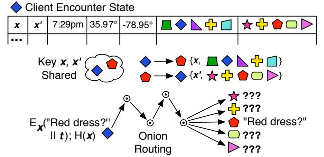
**Figure 7: Distributed scheme operation. During an encounter, each peer shares  $k$  identifiers and an encounter key. Messages are sent using onion routing or an anonymous remailer to preserve anonymity.**
