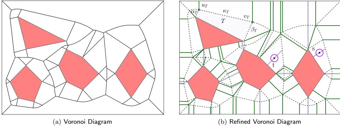
Figure 1: Voronoi diagram and Refined Voronoi diagram of a set of obstacles (dark red). (a) Voronoi edges depicted by solid black lines. (b) Voronoi edges depicted by dashed black lines, Green solid lines and blue dotted lines represent type (i) and type (ii) edges, respectively. Lines through  $s$  and  $t$  represent type (iii) edges. A representative cell  $T$  depicted in light blue.
