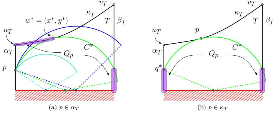
Figure 9: Case 2 of proof of Lemma 4.6. Green circle  $C^*$  which intersects  $p$  centered at  $(x, 0)$  and tangent to  $\kappa_T$  defines the points  $Q_T$  (purple) visible to  $p$ . (a) Circles intersecting  $p$  centered at  $(x, 0)$  with larger (blue) and smaller (cyan) radii than  $C^*$ , respectively.
