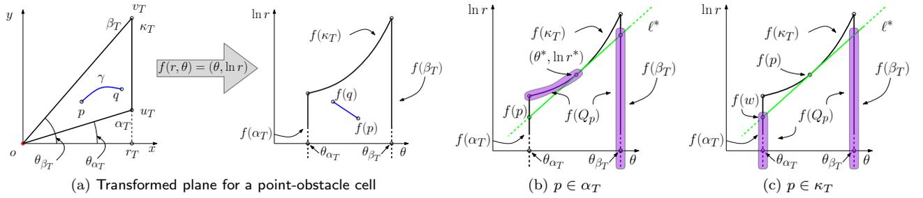
Figure 8: Case 1 of proof of Lemma 4.6. (a) A cell of a point obstacle in  $\tilde{\mathcal{V}}$  and the optimal path between points  $p$  and  $q$  (blue) in the original (left) and transformed plane (right), respectively. (b,c) The set of visible points  $Q_p$  (purple) to the point  $p$  in the transformed plane.
