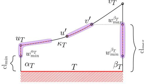
Figure 6: Samples placed on the edges of a cell  $T$  of  $\tilde{\mathcal{V}}$ . The sampled regions are depicted in purple. For the constant-factor approximation algorithm, samples are placed on  $\beta_T$  only.
