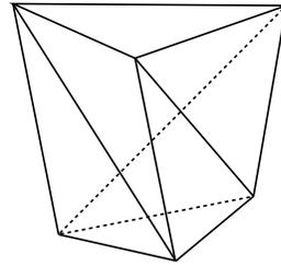
Figure 4: A polyhedron that cannot be triangulated without Steiner points.
