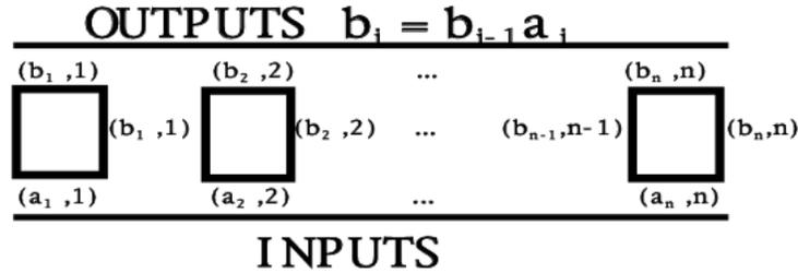
Figure 5: 2D assembly for sequential prefix computation.
