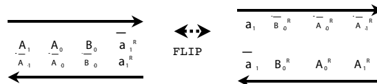
Figure 14. A duplex resulting from full hybridization of the DNA fuel strand with the wheel, and a flip of the duplex.
