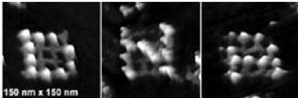
Figure 18: 2D Patterns by hierarchical assembly AFM images of characters D , N , and A .
