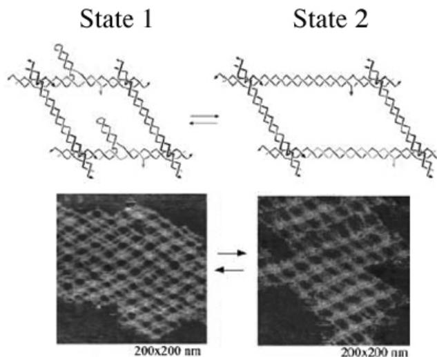
**FIGURE 5** *Upper panel:* Schematic drawing of the two states of the lattice unit structure. *Lower panel:* Representative AFM images of the rhombus lattices displaying different morphologies, which can be reversibly switched by the DNA nanoactuator.
