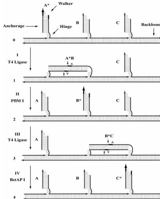
**FIGURE 6** The structural design and operation of the autonomous unidirectional device. The bold fragments are the walker fragments. The arrows indicate the PflM I and BstAP I restriction sites. The curves indicate the ligation sites.
