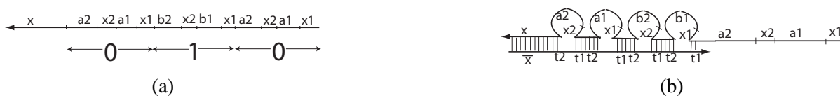
Figure 4: (a) Encoding of 0 and 1 in DNAzyme FSA. (b) Protector strand partially hybridizes with the input strand to form bulge loops. The sticky end formed at the end of the input strand outside of the bulge loops represents the active input symbol. This scheme protects the input symbols other than the currently active symbol from becoming active.
