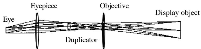
Figure 5-(i). Paraxial model layout at position 1
