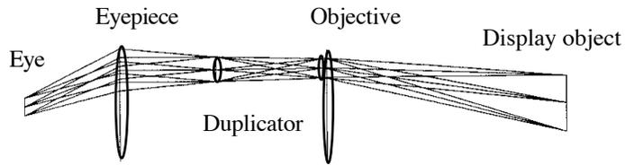
Figure 5-(ii). Paraxial model layout at position 2
