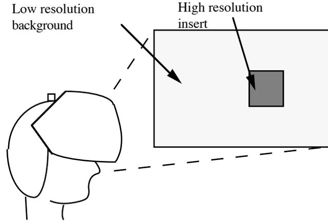
Figure 1. High resolution insert HMD
