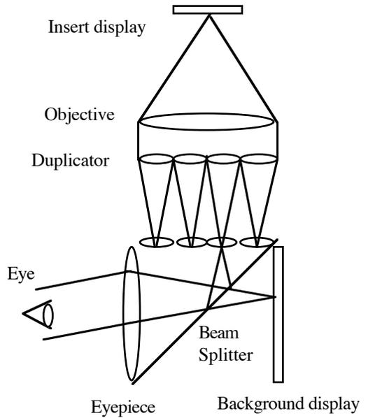
Figure 3. Schematic Diagram of the HMD
