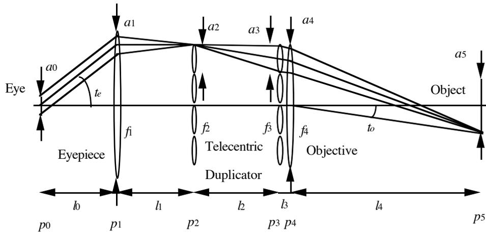
Figure 4. System parameters of the HMD
