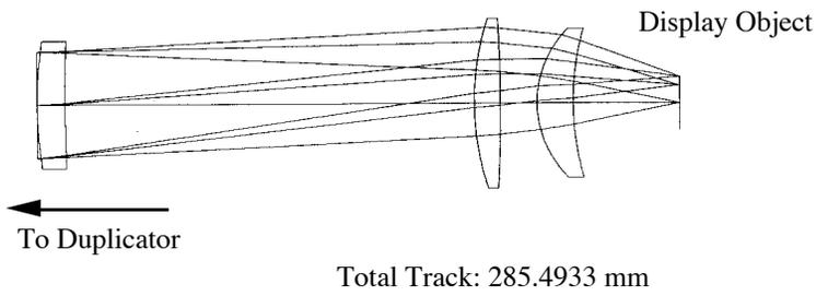
Figure 8-(i). Objective layout
