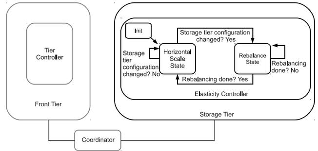
**Figure 5: Block diagram of the control elements of a multi-tier application. This diagram shows the internal state machine of the elasticity controller of the storage tier, but depicts the application tier as a black box.**
