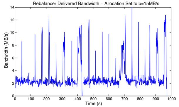
**Figure 3: Delivered bandwidth of the HDFS rebalancer (version 0.21) for  $b=15\text{MB/s}$ . Although the bandwidth peaks at the configured setting  $b$ , the average bandwidth is only 3.08MB/s. We tuned the control system for the measured behavior of this actuator.**
