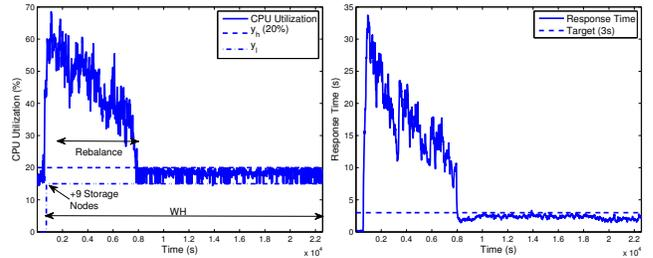
(c) Average CPU utilization of the HDFS datanodes with dynamic provisioning
