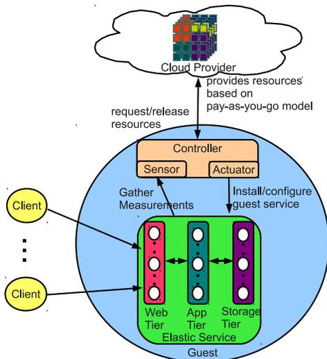
**Figure 1: A multi-tier application service (guest) hosted on virtual server instances rented from an elastic cloud provider. An automated controller uses cloud APIs to acquire and release instances for the guest as needed to serve a dynamic workload.**
