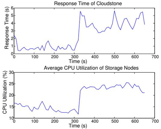
**Figure 2: Cloudstone response time and average CPU utilization of the storage nodes, under a light load and a heavy load that is bottlenecked in the storage tier. CPU utilization in the storage tier correlates strongly with overall response time (the coefficient is .88), and is a more stable feedback signal.**
