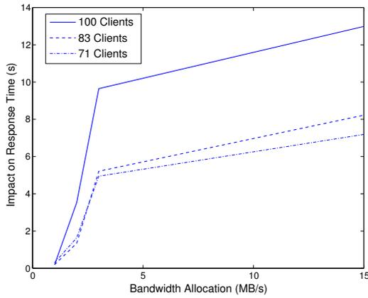
**Figure 4: The impact of HDFS rebalancing activity on Cloudstone response time, as a function of the rebalancer’s bandwidth cap and the client load level. The effect does not depend on the cluster size  $N$  because the cap  $b$  is on bandwidth consumed at each storage node.**
