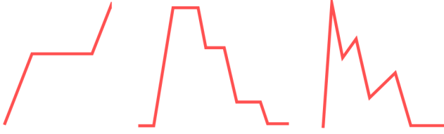
Fig. 1. The number of extrema of a sampled function can be drastically different from the number of zeros of its discrete gradient. From left to right: the signals have no extrema, 1 local maximum, 3 local maxima and 2 local minima, respectively. The definition of a local extremum is in Section 2.
