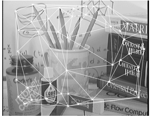
Figure 5: The first frame used in the experiment, with the Delaunay triangulation of the selected features.
