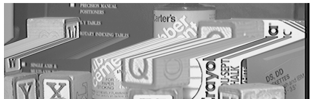
Figure 6: An epipolar slice (center) sandwiched between the top of the first and bottom of the last frame of a 50-frame image sequence.
